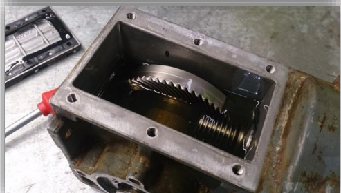
Visual inspection of the oil and any contamination.
