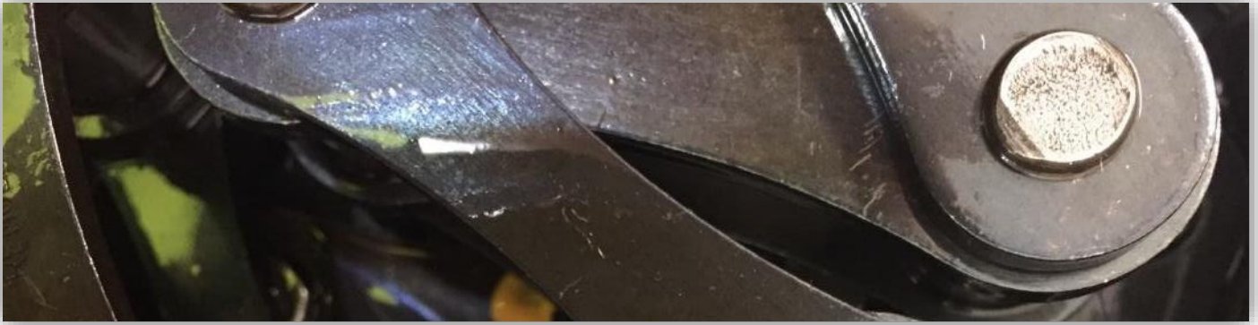
New chain with grease / oil preservative
