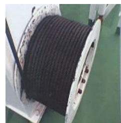
Buy dry cables and lubricate with Fin Lube EP.
