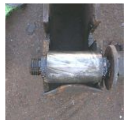
After six months of exposure to the elements and occasional periods of three weeks under water, the pin and bearings still look good and show no signs of wear.
