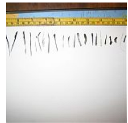
Metal debris caused by wear.
