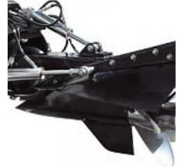
Tunnel prop drive.
