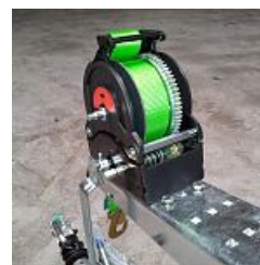
Interflon Fin grease for lubricating the cogwheels.
